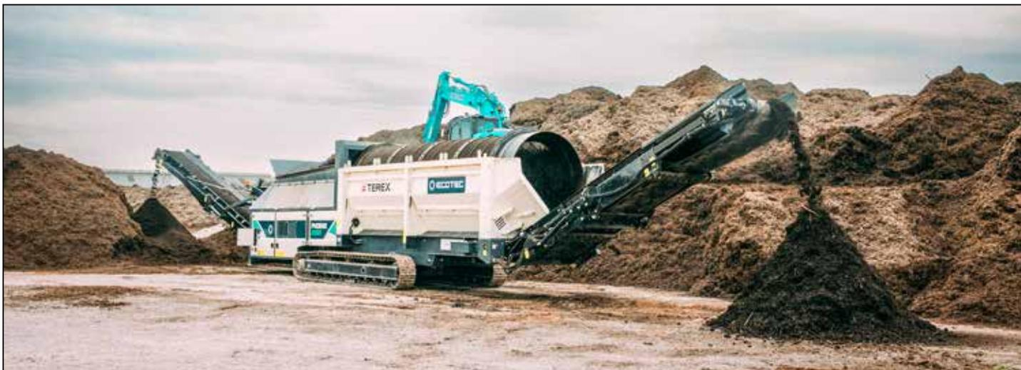
Terex Ecotec has further enhanced its trommel offering with the launch of the new Phoenix 2100T—a tracked variant of the market-leading Phoenix 2100 Trommel. The 2100T has been intuitively designed offering operators unrivalled throughput, application flexibility and serviceability.
